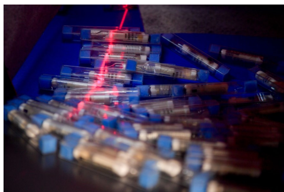
Laser scanning identification code during fully automated storage of ampoules with freeze-dried bacteria. Photo credit: DSMZ
